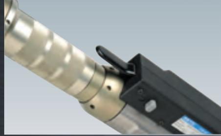
Push the lever to activate the tool, and release it to stop.
